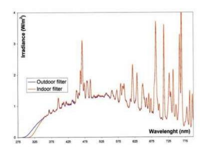
A complete range of advanced UV filters are available to match sunlight conditions: direct exposure to sunlight (Outdoor); exposure through a window glass (Indoor); Outdoor and Indoor filters with IR coating to reduce infrared radiation on samples.
