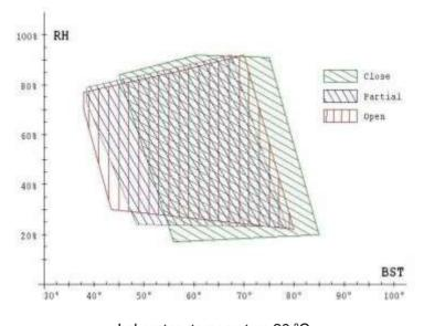
Blue range is for partially closed air circulating circuit. Red range is for fully opened air circulating circuit
