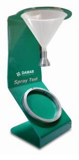
This instrument allows the operator to do water repellency tests to determine the behaviour of a fabric or leather to absorb water that get in contact with the same, in form of rain.
